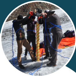
Ice core drilling at Machoi
